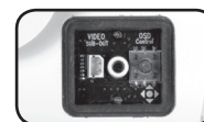
Secondary Video Output & OSD Control Joystick are accessible inside a Gasket sealed removable side panel.
