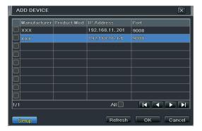
③ Checkmark the device you want to add and then click "OK" button to return to the previous interface to apply the settings. Status will display "Connected" if successful and will display live image. You may select the added device and click "Setup" button to modify channel, IP address as shown in Fig 5.
