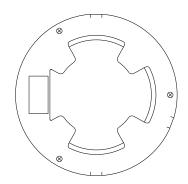
Route the cables and connect the power & video cables, then secure the mounting base to the ceiling or wall with screws.
