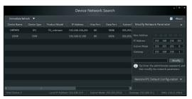
3. Modify the IP address. The default IP address is 192.168.226.201. Click the information of the camera listed in the above table to show the network information on the right side. Modify the IP address and gateway of the camera and make sure its network address is in the same local network segment as the computer's. Please modify the IP address of your device according to the practical situation.
