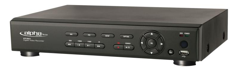
The Alpha Series VT-H41 Digital Recorders combine the latest H.264 Compression technology with stability and simple operation. H.264 Compression is the next generation of MPEG4 allowing up to 50% smaller file sizes for increased storage capability and/or resolution as well as a more fluid internet transmission speed. Either unit can be controlled via supplied IR Remote control or remote client. Convenient front panel controls are included.
