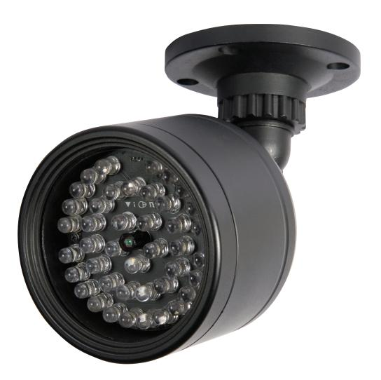
The VT-IR42/24 Infrared Illuminator is designed to enable your B/W CCD camera to deliver useable images in absolute darkness. It has range to 50 feet and runs off of low voltage 24 VAC (the same as most surveillance cameras). Heavy-duty aluminum construction and condensation-free design enable usage indoor and outdoors. IR protecting technology prevents LEDs from overheating and extends the lifespan to its maximum.
