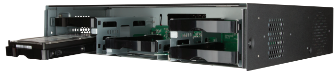
Easy to load HDD with removable faceplate.
