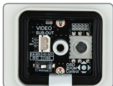
Secondary Video Output & OSD Control Joystick are accessible inside a gasket sealed removable side panel
