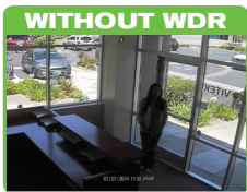
Over/Under Exposure & Poor Color Quality
