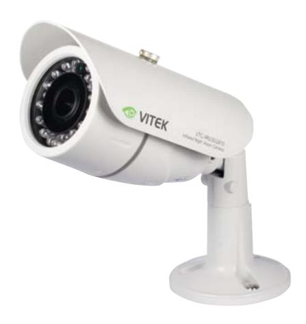
The VTC-IRV30/2810 is a Weather Resistant, self enclosed bullet style IR camera with a 2.8-10mm adjustable focal length auto iris lens. This attractive, compact and economical camera features a Sony Super HAD CCD with 550 TV Lines of Horizontal resolution, 30 Infrared LEDs with range beyond 100', feed-through wiring, Dual Voltage 12VDC/24VAC operation, and included sunshield.
