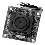
These cameras are easily installed in covert objects and work well in low light conditions. Because they are DC powered, they can be used for mobile applications.
