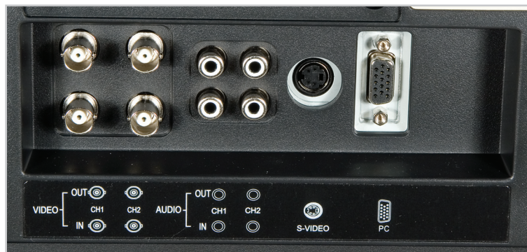
VTM-LCD193P Rear Connections:
